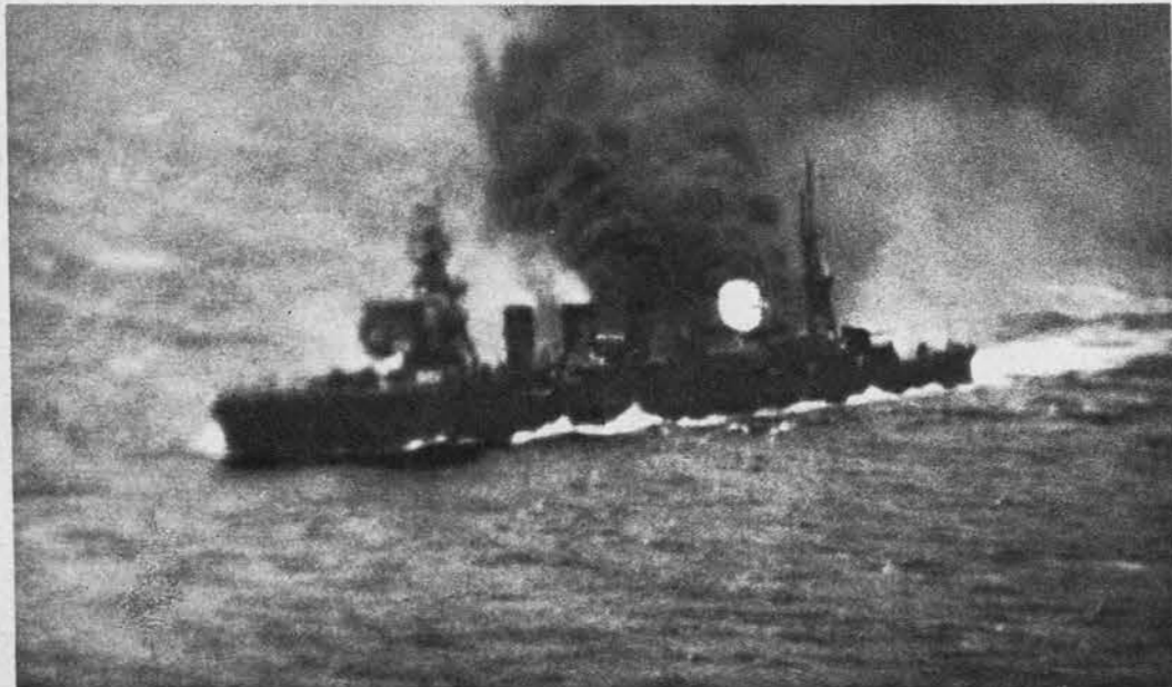
Burning Natori Class ship has broken deck, three stacks, and single shield mounts typical of the older Japanese light cruisers. Kuma Class is similar in general appearance, but with lower bridge.
